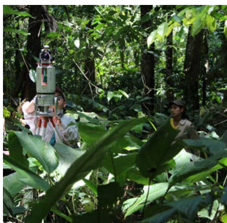
Setting up Terrestrial LiDAR Scanner for capturing tree structure in peruvian amazon forest. Photo: Alvaro Lau Sarmiento
