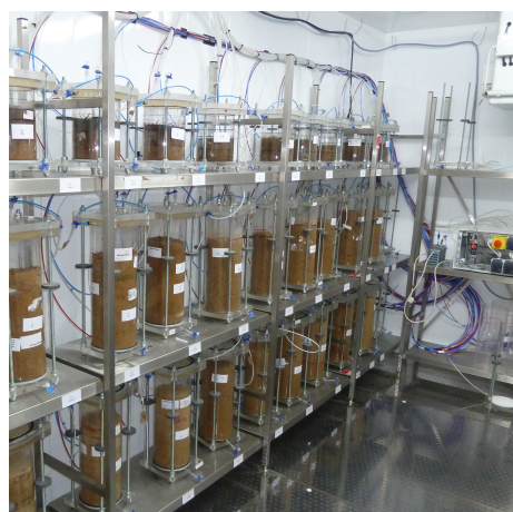
Soil mesocosm incubation system for continuous monitoring of gaseous fluxes at the Thünen Institute. Photo: Wordell-Dietrich
