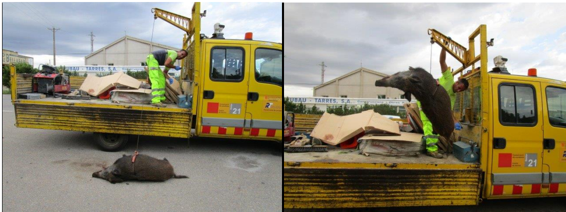
Figure 5.30. Trucks adapted to remove large animal carcasses from roads and roadsides are being used in some countries to improve the management of the large number of ungulates that should be appropriately processed. Photo: Catalan Government-Department of Transport and Sustainability.
