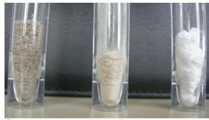
Struvite precipitates from different processes
