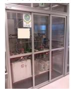
Environmental Technology with an anaerobic hood, two microscopes (one stereo) equipped with a digital camera and connected to a computer for imaging analysis, and equipment to flush headspaces and to create specific headspace compositions in batch tests.
